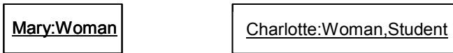
Fig. 2.3. Graphical representation of a classification into entity types. Mary and Charlotte are instances of Woman . Charlotte is an instance of Student too
